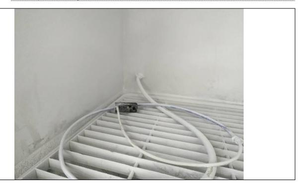
Details of: Internal view of product after IP5X test
